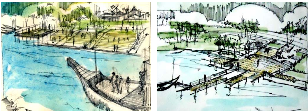
Figures 15-16: Riverbanks can be stabilized with permanent stairways and landing stations to provide adequate spaces for landing and anchorage
