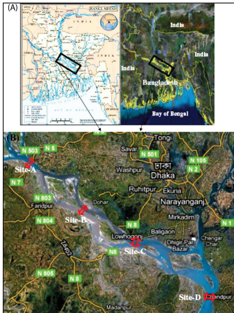
Figure 1: Study area and four potential crossing locations of the Padma River Bridge. (A) A section of the Padma River is marked which indicate inset and is presented at bottom (B). The red double arrows are showed at four potential crossing locations for the Padma River Bridge. The base map is prepared from google earth.
